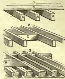
1. A, A, joists; B, floor-boards. 2. C, D, D, binding-joists; E, E, bridging-joists; B, floor-boards. 3. Joists.
